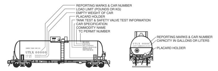
**CAUTION:** Emergency response personnel must be aware that rail tank cars vary widely in construction, fittings and purpose. Tank cars could transport products that may be solids, liquids or gases. The products may be under pressure. It is essential that products be identified by consulting shipping documents or train consist or contacting dispatch centres before emergency response is initiated.
